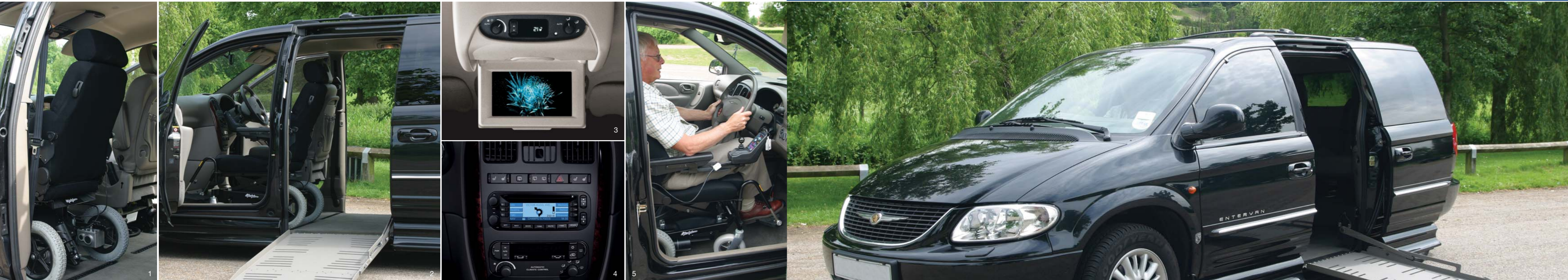
6 & 7 - Operation of the door, ramp and suspension by the original Chrysler remote key fob. With the suspension lowered, the angle of the ramp can easily be negotiated by a manual wheelchair. 8 - Entering the vehicle via the ramp. The ramp can be fitted to the left or right of the vehicle. 9 - A wheelchair shown secured by manual webbing system. 10 - A wheelchair passenger can travel in the front next to the driver, no more shouting from the back of the vehicle. 11 - The vehicle can be driven from the wheelchair.
